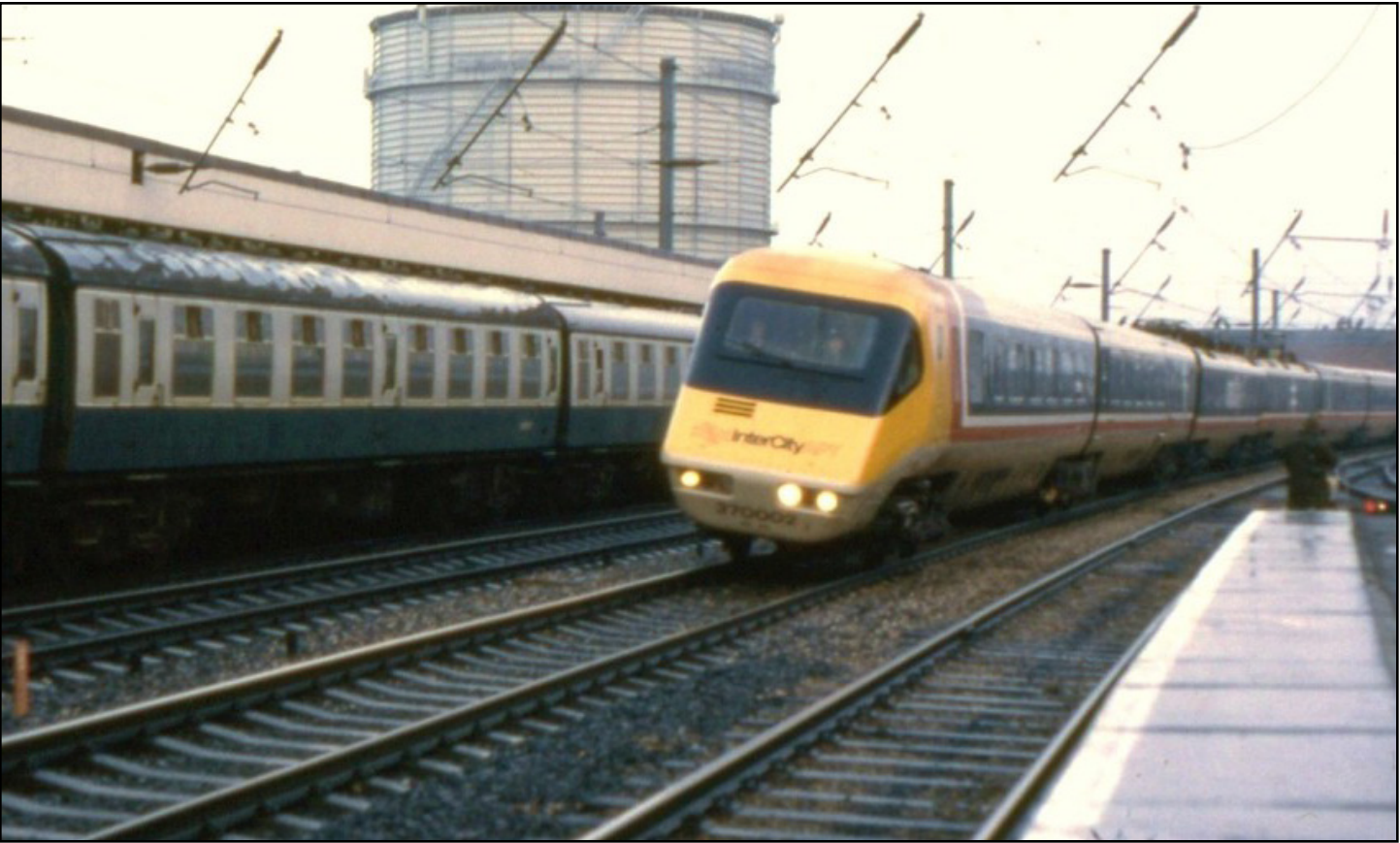
Mocked in its time, British Rail’s Advanced Passenger Train (APT) pioneered the tilting technology that underpins Amtrak’s Acela.
