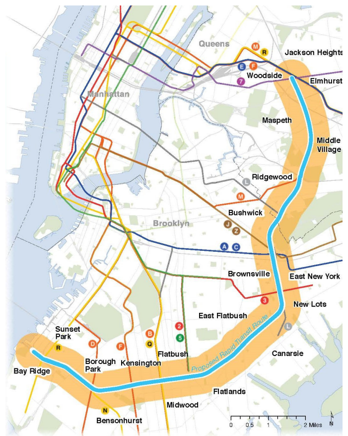
Overview map of the existing freight rail corridor, subway connections, and the primary study area. Note that while most of the IBX corridor runs along the Bay Ridge Branch, a portion includes the Fremont Secondary.
