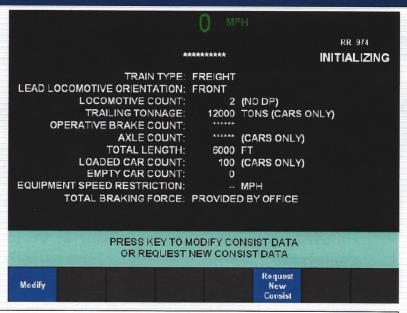
During Initialization, the Onboardwill receive and display the summary consist information to the locomotive operator with a prompt "PRESS KEY TO MODIFY CONSIST DATAOR REQUEST NEW CONSIST DATA". This is an indication that there are items that need to be modified. In addition, another indication would be asterisks noted in the body of the Consist Summary. The locomotive operator would need to select the "Modify" key, make changes and then select the "Accept" key ifavailable.
