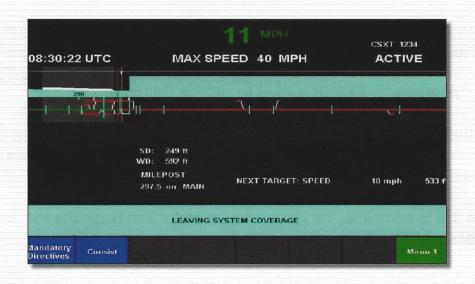
The system will display a "Leaving System Coverage" banner anytime the train moves from PTC track to Non-PTC track. Crew will receive this banner upon exiting PTC track. EXAMPLE: "Leaving System Coverage" may indicate that a hand operated switch is lined for a movement away from the main line.
