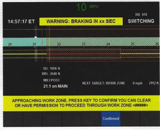
An additional confirmation has been added to the PTC work zone prompts. Should a train be required to enter or move inside working limits within 30 minutes prior to the effective time, the locomotive operator will receive the following prompt. "Press key to confirm you can clear or have permission to proceed through work zone."
