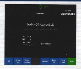
If after completing Initialization, the On-Board Unit cannot determine the train's current location, the OBU will indicate "MAP NOT AVAILABLE". This is an indication that the locomotive operator must manually select the train's location by pressing the "Menu 1" key. The locomotive operator will then select the "Select Location" key.
