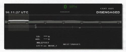
A movement of 30 to 80 feet must be made to transition into Active state.
