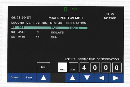
When required to add a locomotive to the consist, locomotive operators must ensure the engine number to be added is preceded by "Null" in the appropriate boxes.
