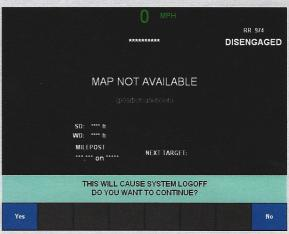
Locomotive operators are required to logoff of the PTC system at the end of their tour of duty. The crew logoff soft key can be accessed by pressing the Menu 1 key.
