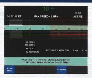
The PTC system will alert the crew within 3 miles of an active Work Zone. The blue banner will remind the crew that verbal permission from the Employee in Charge needs to be obtained prior to entry into the work zone. A red hash box provides protection at the beginning of the workzone.
