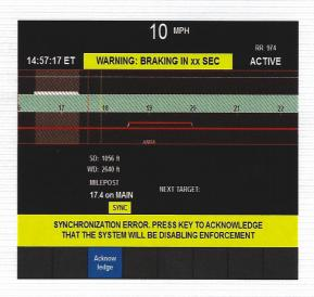
Locomotive operators are required to answer Synchronization Error prompt when displayed on the PTC screen. Locomotive operators should press the "Acknowledge" soft key when displayed. If the soft key is not pressed within the warning timeframe, PTC will initiate an enforcement
