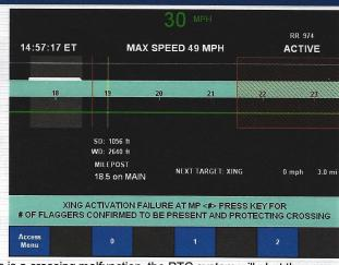
If on train messages or upon receiving EC-1 directive that there is a crossing malfunction, the PTC system will alert the crew prior to arrival at the indicated crossing, by displaying a red hash box, notification banners and "Yes" and "No" soft keys.
