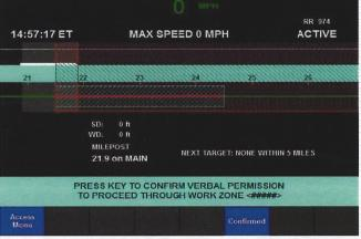
If required to stop either within or approaching an active work zone, PTC will prompt the crew for permission to continue through the work zone prior to the train moving. Previously, trains had to begin moving in order to get prompted for permission to continue through the work zone. If movement is made prior to answering this prompt, train will be enforced.
